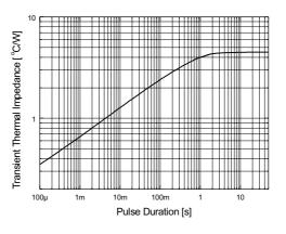
Figure 4. Thermal Impedance Characteristics
