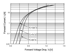
Figure 1. Typical Forward Voltage Characteristics
