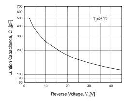
Figure 3. Typical Junction Capacitance
