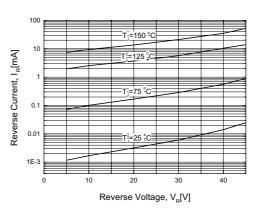
Figure 2. Typical Reverse Current vs. Reverse Voltage
